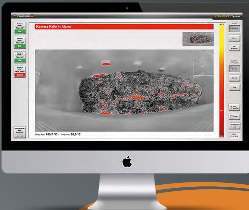
*Panoramic thermal imaging: View of a waste bunker with patented abiroVision® software*
